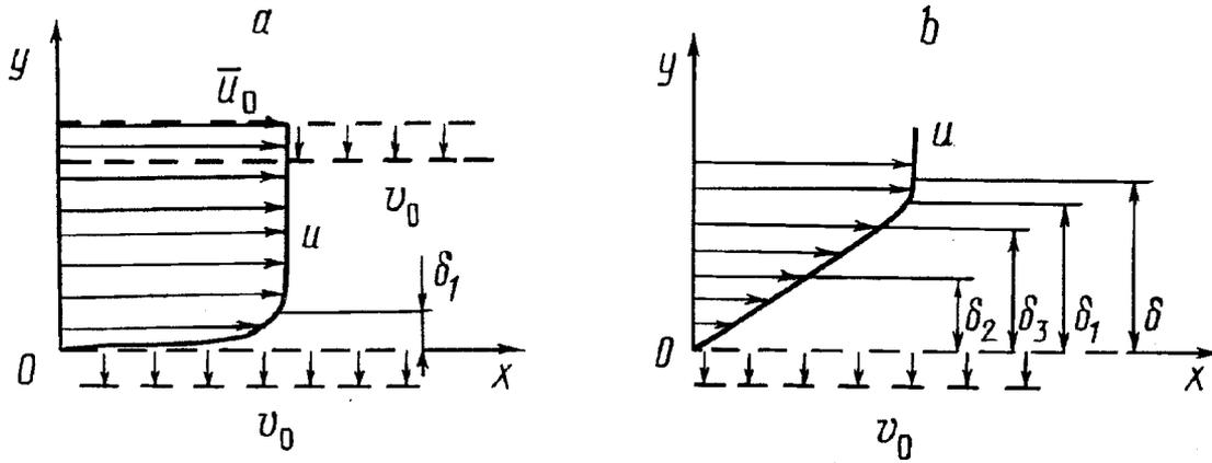
Fig. 2. Flow of a viscous liquid between moving horizontal permeable planes (a) and in the boundary layer (b).
