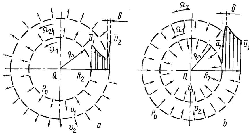
Fig. 1. Flow of a viscous liquid between rotating coaxial permeable cylinders of infinite length with a source (a) or sink (b) linearly distributed along the axis.
